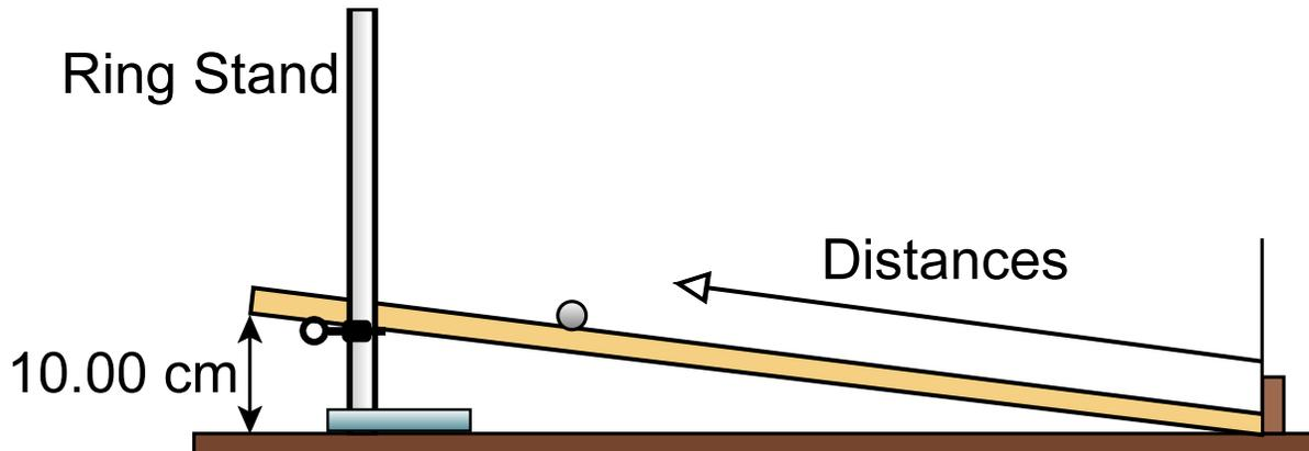
Use the ring stand and ring to raise one end of the track until the distance between the bottom of the track and the tabletop is 10.00 cm.
